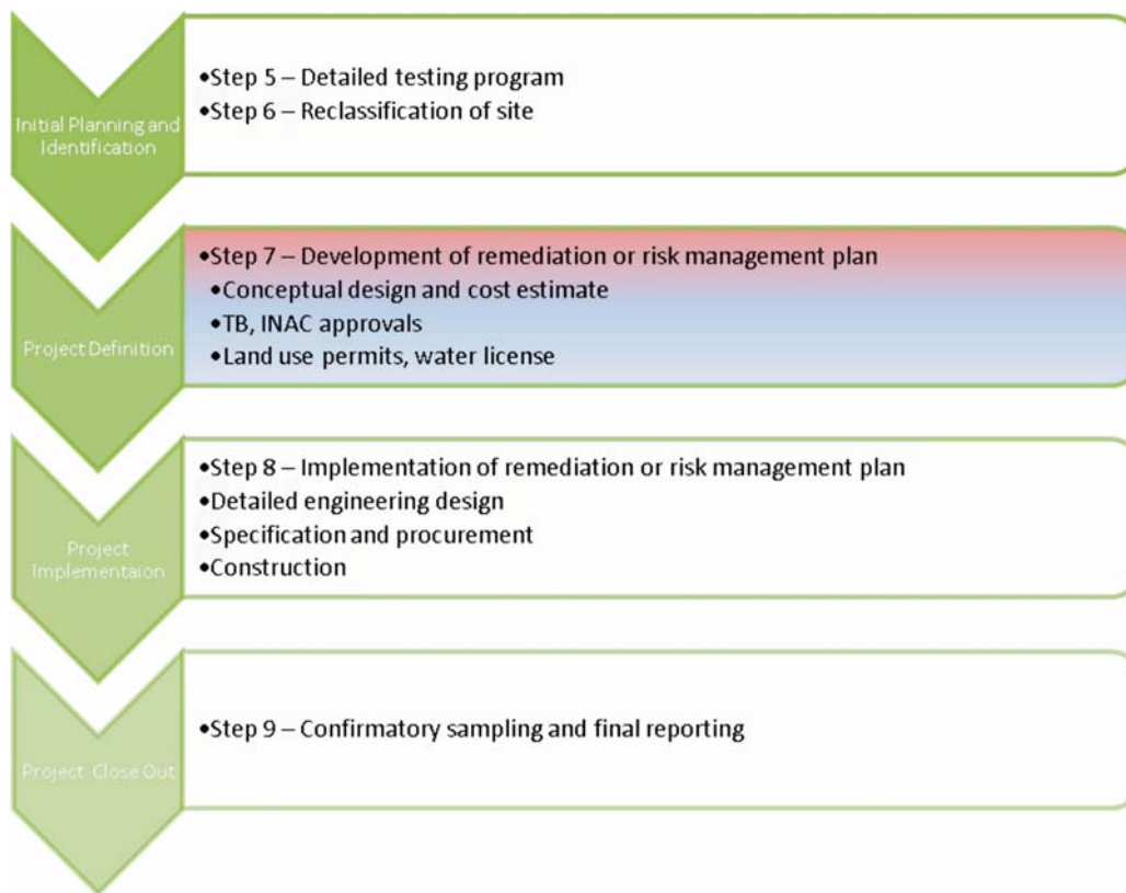
Figure 1: Main phases of contaminated-site remediation within the context of the Northern Contaminated Sites Program.
